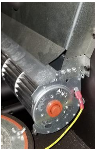
N130WTS N60WTS, NBF66WTS Figure 21 Convection Blower Disassembly
