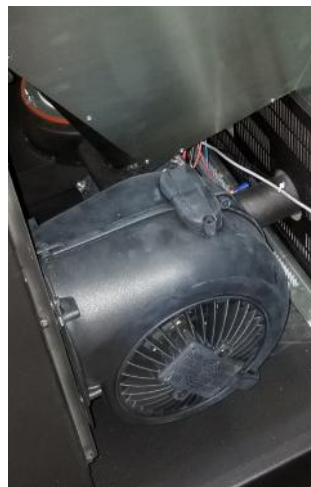
N130WTS N60WTS, NBF66WTS Figure 21 Convection Blower Disassembly
